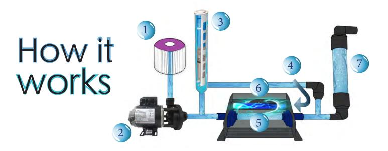
Contaminants and large particulates are first trapped by the *Microfilter*.
